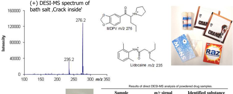
Analysis of powdered samples for DESI-MS via Teflon filters
