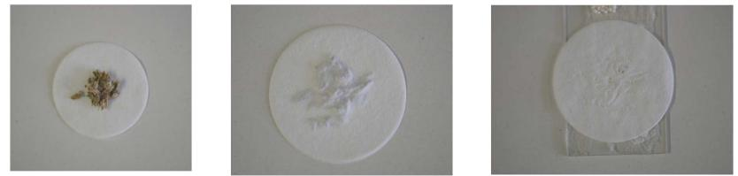
left: Spice product on teflon filter; middle: Spice product pressed between two teflon filters; right: teflon filter on glass slide for für DESI-MS (second filter optionally for IMS)
